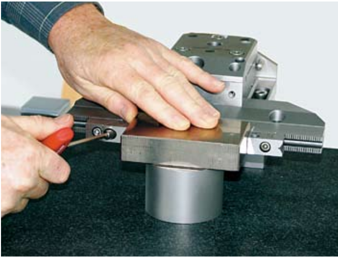
1. Clamp the workpiece in the holder
