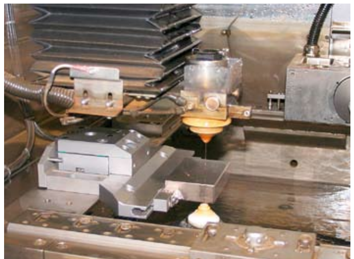
3. Erode the workpiece
