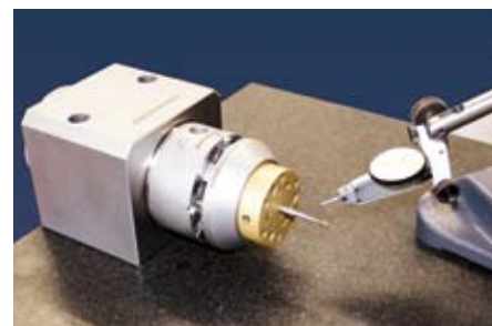
Presetting with Presetting Spindle and Adjustable Clamping Element
