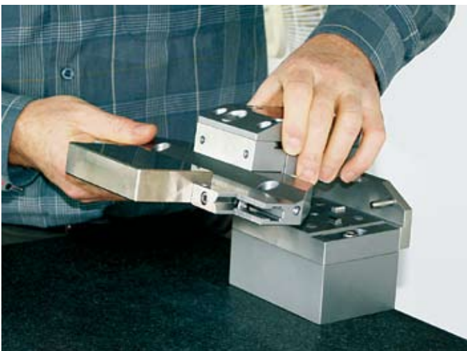
3. Withdraw presetted workpiece
